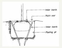
Use untreated wood stakes inserted 4 stakes along the outside of the rootball. Drill two stakes horizontally across the vertical stakes along the top of the rootball to stabilize the rootball, but still allowing the tree to have movement. The stakes will decompose over time and the tree will grow structurally stronger.
